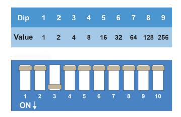
Unique or Shared Addressing: If all fixtures share the same profile (e.g., all are 3-channel RGB fixtures) and individual control is not required, it is possible to set the fixtures to the same DMX address. Otherwise, individual fixture control requires that each fixture be set to a unique address and that no DMX fixture channels overlap.
